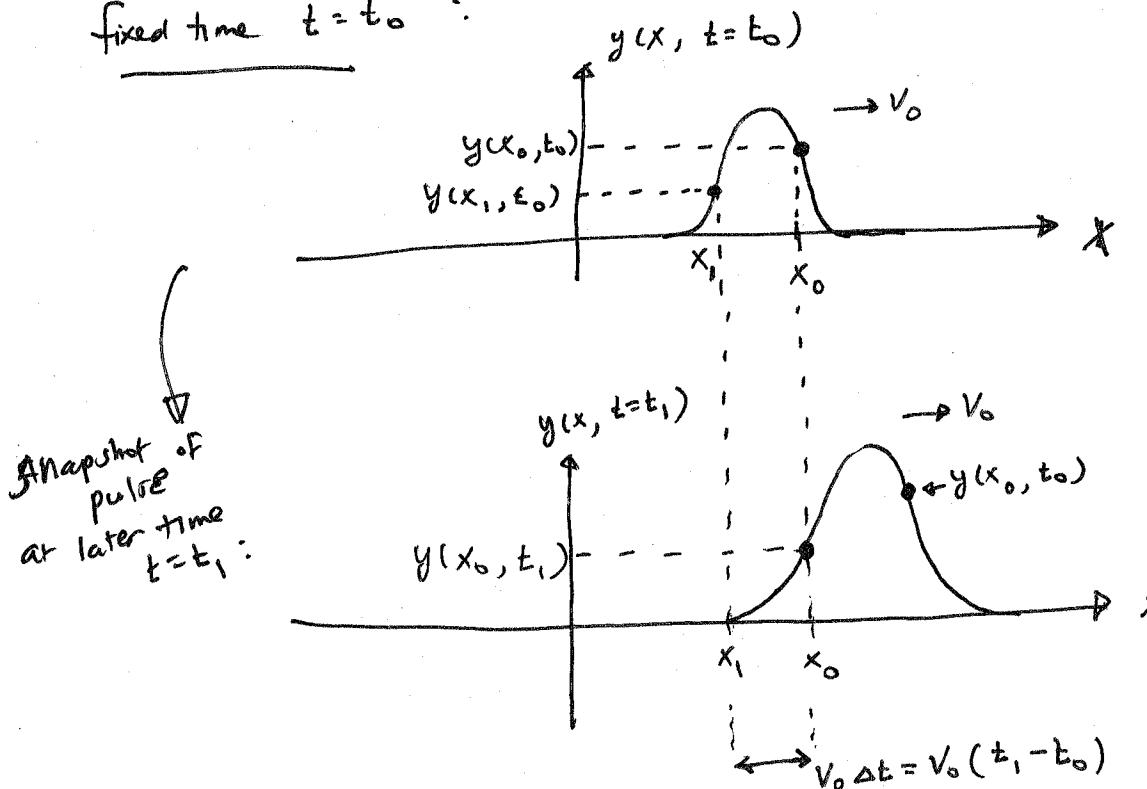
Thus,  $y(x_0, t_0) = y(x_0, t_0)$  but  $x_1 = x_0 - v_0(t_1 - t_0)$
