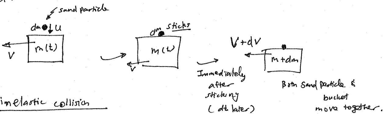
This is an inelastic collision.
