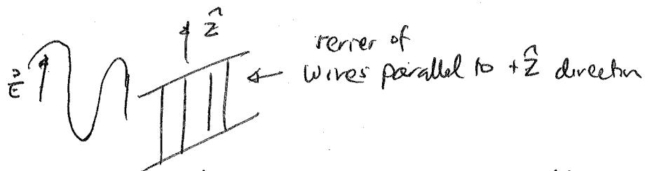
Component of  $\vec{E}$  vector that's parallel to the wire ( $\vec{z}$ -axis is this case) blocked out since it drives free  $e^-$  along the wire.
