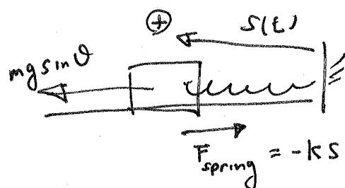
$$\begin{aligned} m \frac{d^2 s}{dt^2} &= m g \sin \theta + F_{\text{spring}} \\ &= m g \sin \theta - k s \\ &= k s_0 - k s \quad \leftarrow \text{from (a)} \\ &= -k(s - s_0) \end{aligned}$$
