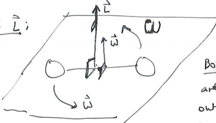
Both  $\vec{\omega}$  and  $\vec{L}$  are vectors pointing out of page, & perpendicular to the page as drawn here.
