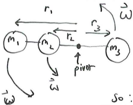
About the pivot, all masses connected by massless rod rotate together with the same angular frequency  $\vec{\omega}$ .
