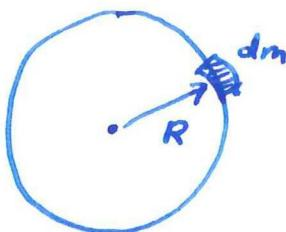
All mass element  $dm$  is located at same distance  $R$  from the center of the circle.
