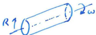
Like the onion ring, all mass element  $dm$  is at distance  $R$  from the axis of rotation.
